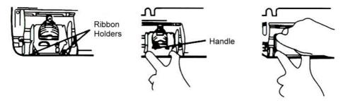
3. Correctly insert a new cartridge between the ribbon guide and the printer head. Push the cartridge head until it clicks into place. Then, turn the knob clockwise to secure the ribbon.
